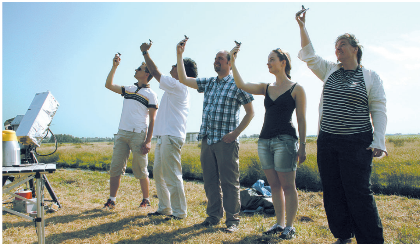
Researchers measure atmospheric aerosols with iSPEX optical devices and smartphones.
